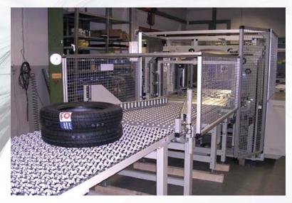
Fully automatic twist wrapping machine for high performance requirements
